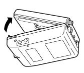
then attach the bottom as shown in Hook the upper catches of EDH-27 in the slots at the top of the DJ-X2, and the illustration on the left.
