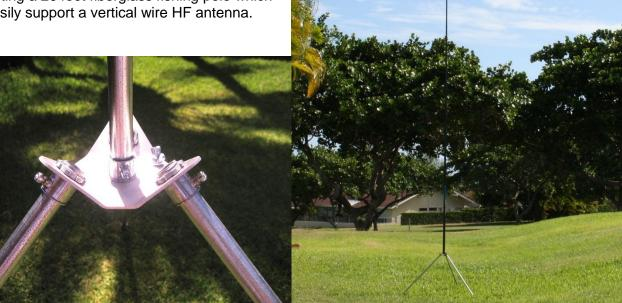
**Assembly of Tripod Plate** The three outer holes accept screw type ½" conduit connectors for the legs, and the center hole accepts a ½" conduit connector to support a 30" section of conduit, which in turn supports the fiberglass pole. The small hole is for a #10 machine screw, hex nut and wing nut, and serves as a counter poise connection point.
