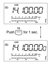
Rotating the tuning dial changes the frequency in 10 Hz steps.
