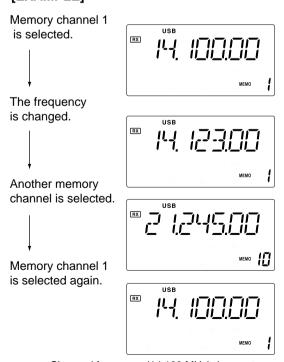
Changed frequency (14.123 MHz) does not appear and memorized frequency (14.100 MHz) appears instead.
