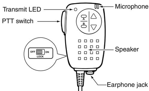
The HM-75A has a lock switch on the backside to prevent accidental frequency changes, etc.
