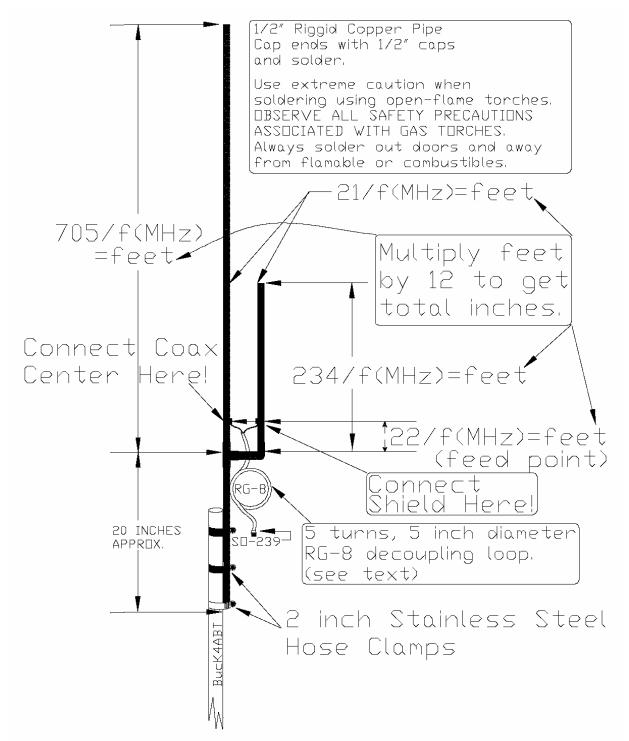
Notice how the decoupling loop is formed from a length of the coax coiled into a 5 turn, 5 inch diameter loop. The coil is then attached it to the mast as shown above. For the final touch, attach an SO-239 (female) coax connector; see text.
