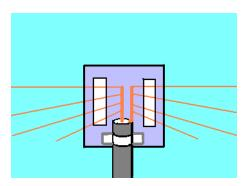
The white areas in the center support drawing above are mechanical supports, clamps, wire ties or whatever your genius can come up with to support the main (top wire) and the weight of the coax. Remember, all the weight of this antenna system is supported by the top wire.
