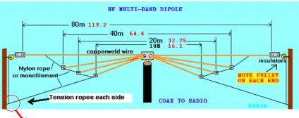
Tension rope is not tied to pully rope in picture. It is tied near location of pully rope down on supports within easy reach. It is tied last after final SWR adjustment and the antenna is in it's final position.
