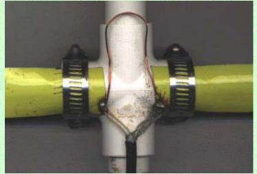
I used 1 1/2 inch hose clamps to attach all the elements
