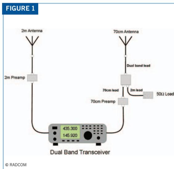
Figure 1: Desensitisation filter using a diplexer.
