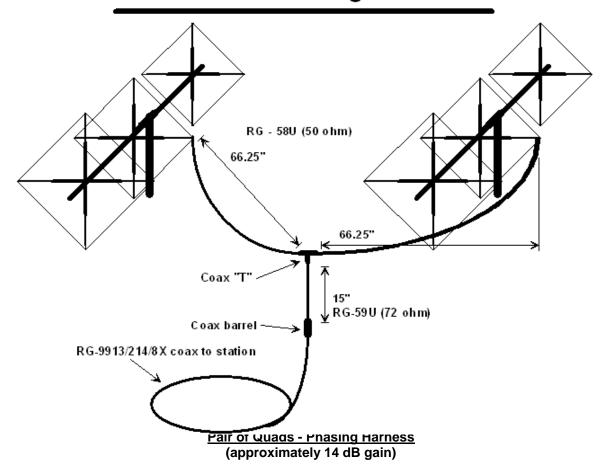
Each leg of coax from the antenna to the first barrel connector is of RG-58 coax with bazooka balun at a length of 66.25 inches each (each leg must be identical) and attached as shown for both antennas to be "IN" phase complementing one another.
