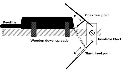
NOTE: Moving the feed point attachment up and down the Quad wires will vary the VSWR. When the construction is completed solder the coax/balun - Quad wire attachment points.
